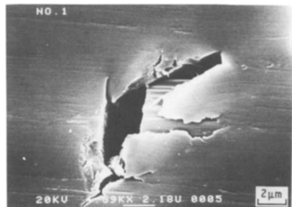
Figure 6 A magnified view of the fibre breakage.
